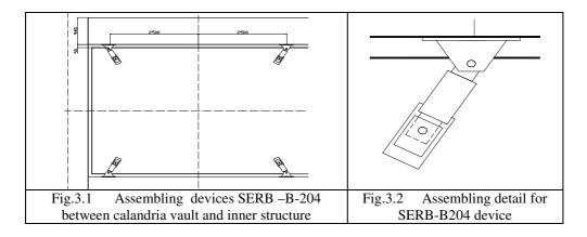
The large damping capacity of the devices including at very small displacements, is improving the overall seismic behavior of the inner structures and Calandria vault by the reduction of the seismic movement amplification.
