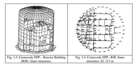
For to evaluate the increase of the safety margin, the analyses regarding the seismic behavior of the inner structures and calandria vault have been conducted in two steps:
