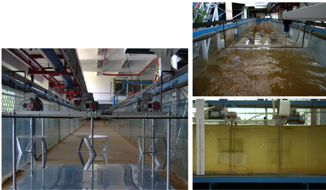
Fig. 1. Experimental set-up: Hydropower farm model at 1:5 scale (left frame); Variable slope open channel (upper-right frame); Turbine models turning in water (lower-right frame)
