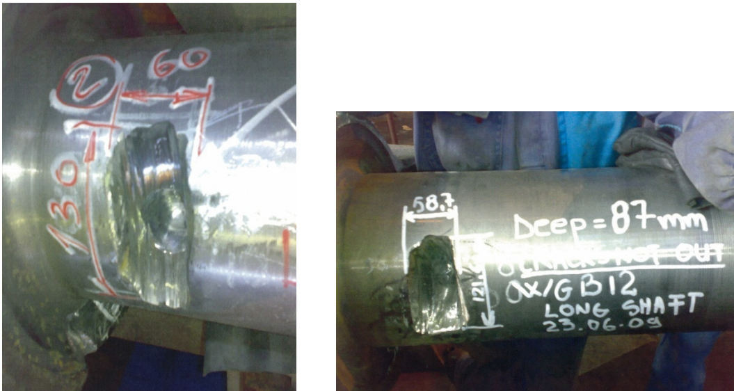
Fig. 6. Excavation on guide vanes long trunnions
