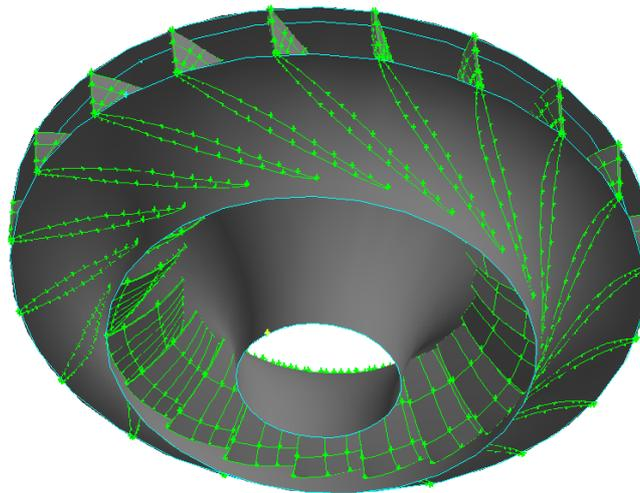
Fig. 2. The three-dimensional geometry of the Francis runner with low specific speed.
