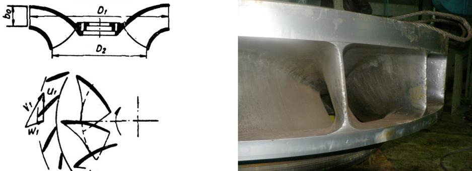
Fig. 1. The Francis runner geometry with low specific speed: sketch (left) and photo (right).
