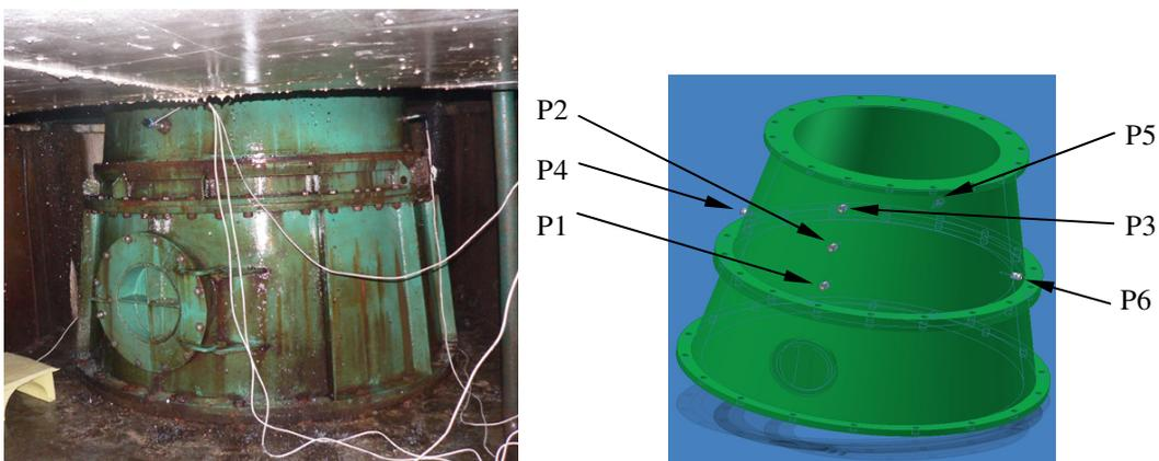
Fig. 6. Photos of the unsteady pressure transducers installed on the cone of Francis turbine prototype with low specific speed (left) and 3D view of the unsteady pressure transducers located on the cone of the draft tube (right).
