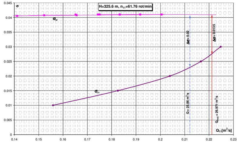
Fig. 5. Thoma cavitation coefficient  $\sigma_{pt}$  (with magenta solid line) and turbine cavitation coefficient  $\sigma_{cr}$  (with brown solid line) of the Francis turbine prototype with low specific speed at nominal constant head.
