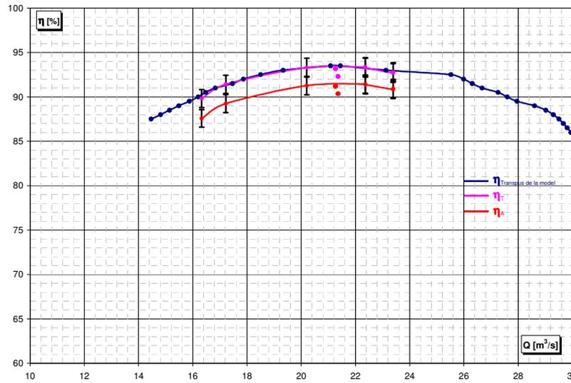
Fig. 4. The turbine hydraulic efficiency  $\eta_T$  computed based on the experimental data (with magenta line) and the hydro unit efficiency  $\eta_A$  (with red line) of the Francis turbine prototype with low specific speed at nominal constant head.
