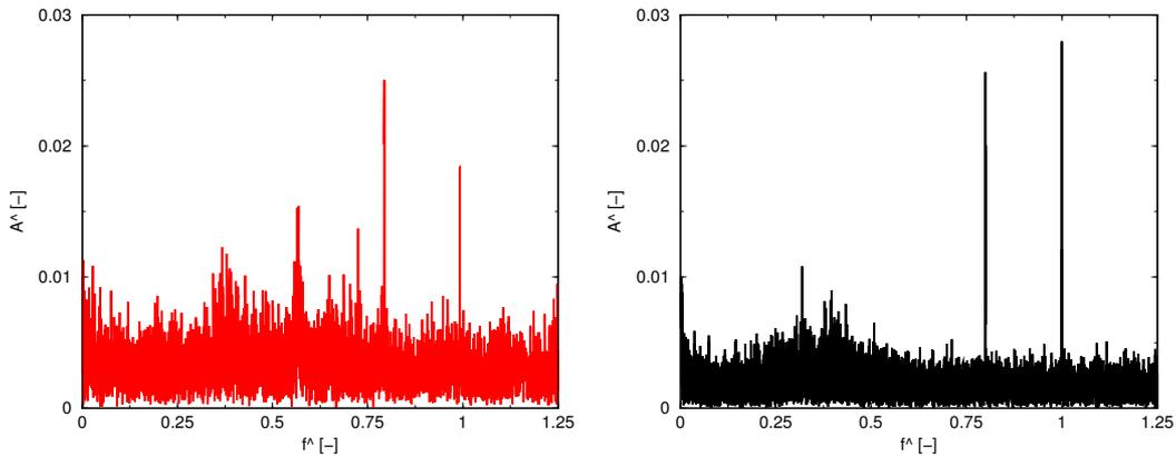
Fig. 7. Fourier spectra of the unsteady pressure transducer P3 installed near to the throat on the cone of Francis turbine prototype operating at 77% partial discharge: without air admission (left) and with air admission (right).
