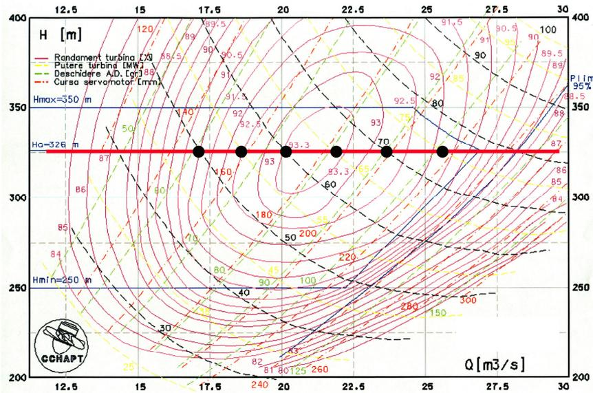
Fig. 3. Hill chart of the Francis turbine prototype with low specific speed. The unsteady pressure was measured on the cone in six points displaced on constant head.
