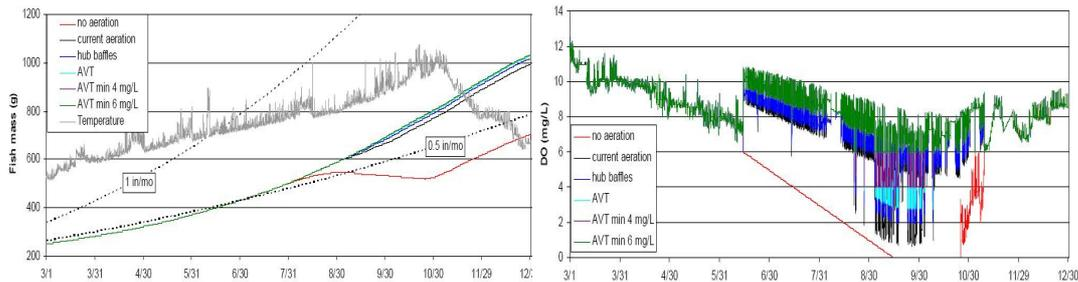
Fig. 3. The results of the model with different aeration scenarios for 1996 (moderate wet year)
