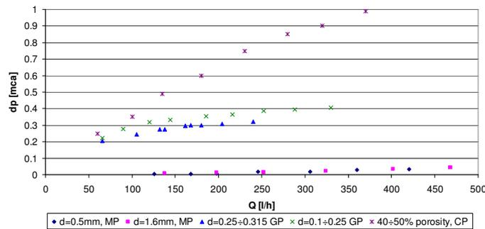
Fig. 5.  $\Delta p = f(Q)$  variation for all the plates tested
