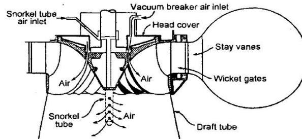
Fig. 4. Aeration through vacuum breaker system and snorkel tube
