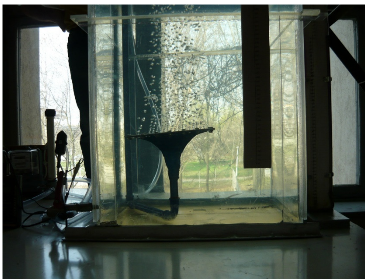
Fig. 1. Fine bubbles generator in function.
