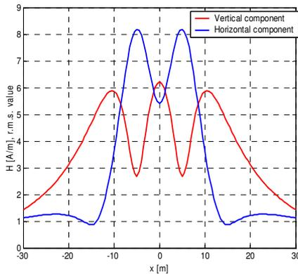
Fig. 11- Magnetic field lateral profile (of axis components) of a 220 kV double-circuit overhead line, with transposed phases, at identical nominal current loads of the two circuits.
