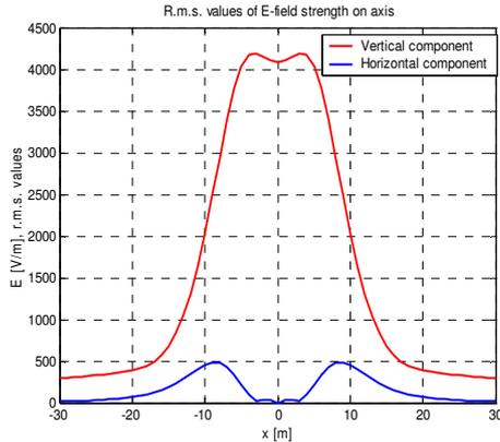
Fig.2- Axis components of electric field produced by a 220 kV double-circuit line with untransposed phases.
