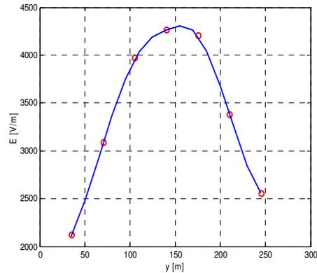
Fig. 8- Electric field longitudinal profile (expressed in r.m.s. values of resultant) of 220 kV double-circuit line, with untransposed phases, with both circuits energized.
