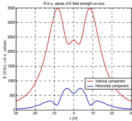
Fig.4- Axis components of electric field produced by a 220 kV single-circuit line; a) tower geometry; b) lateral profile of electric field.
