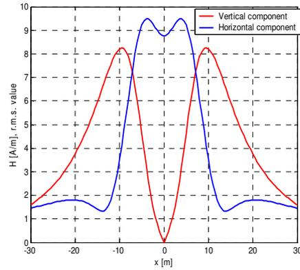
Fig. 10- Magnetic field lateral profile (of axis components) of a 220 kV double-circuit overhead line, with untransposed phases, at identical nominal current loads of the two circuits.
