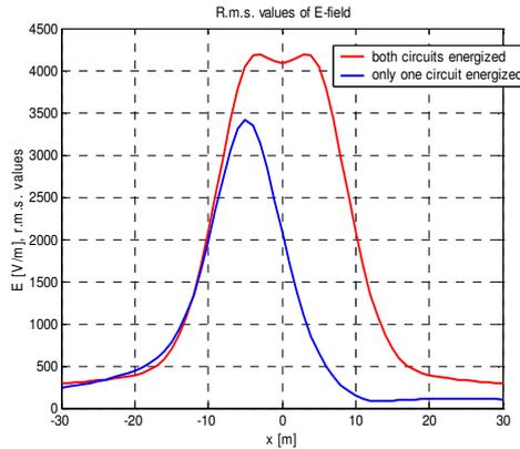
Fig. 5- Electric field lateral profile (expressed in r.m.s. values of resultant) of 220 kV double-circuit line, with untransposed phases, with both or a single circuit energized.
