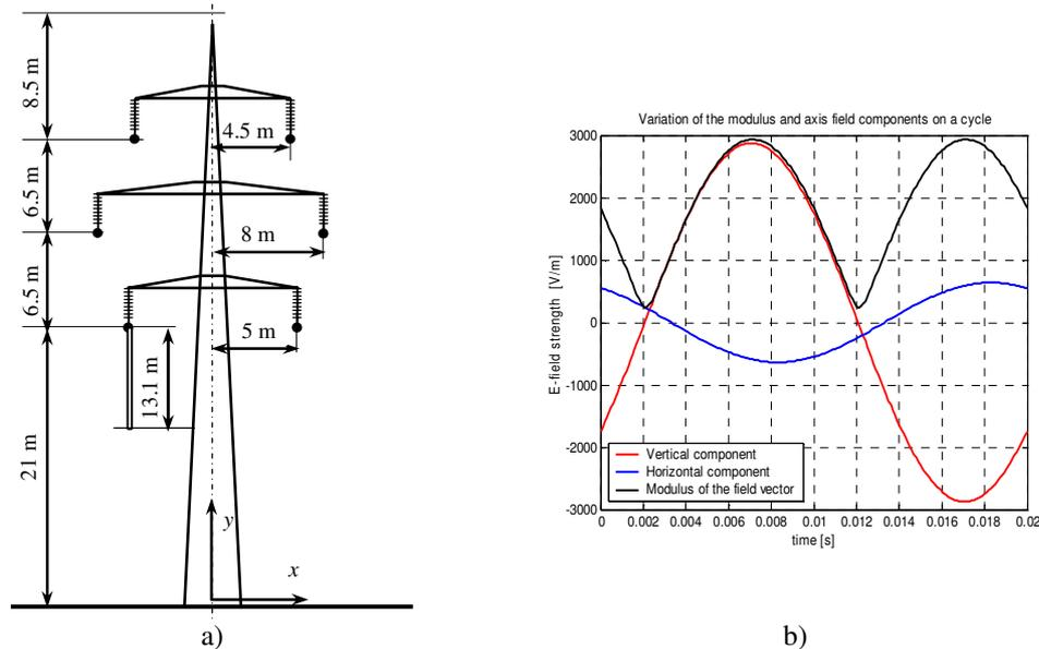
Fig.1. Sketch of a tower for 220 kV double-circuit line (a) and time variation of electric field components on axis and elliptic vector modulus (coordinates of calculation point:  $x=10$  m,  $y=1$  m).
