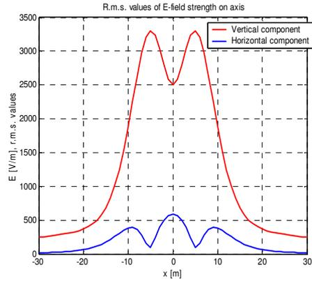
Fig.3- Axis components of electric field produced by a 220 kV double-circuit line with transposed phases.
