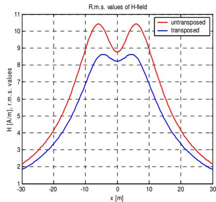
Fig. 12- Magnetic field lateral profile (of axis components) of a 220 kV double-circuit overhead line, with transposed and untransposed phases, at identical nominal current loads of the two circuits.
