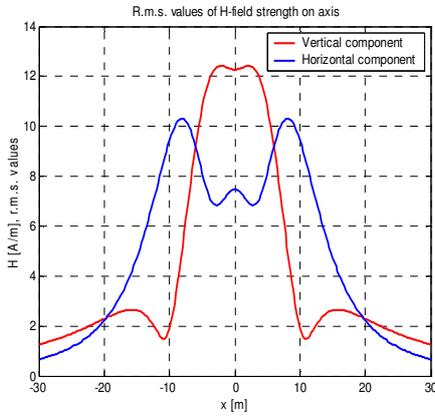
Fig. 9- Magnetic field lateral profile (of axis components) of a 220 kV single-circuit overhead line.
