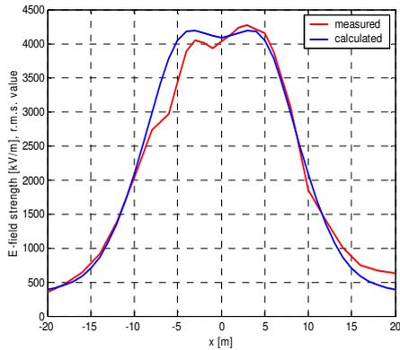
Fig. 7- Electric field lateral profile (expressed in r.m.s. values of resultant) of 220 kV double-circuit line, with untransposed phases, both circuits being energized: calculated and experimental data.
