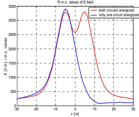
Fig. 6- Electric field lateral profile (expressed in r.m.s. values of resultant) of 220 kV double-circuit line, with transposed phases, with both or a single circuit energized.
