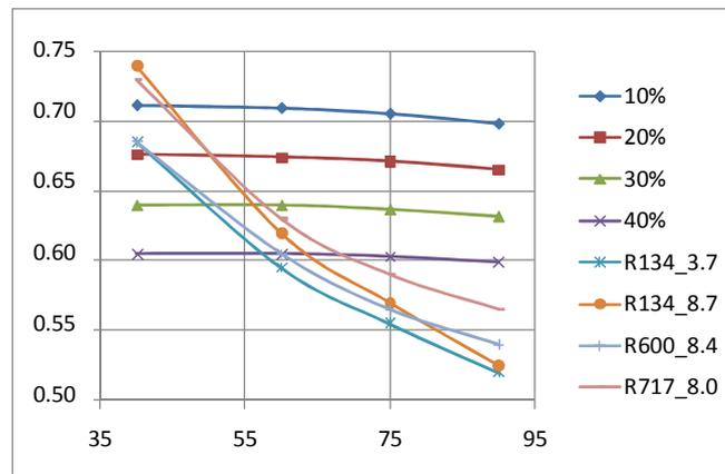
Fig. 4. Overall efficiency of power + thermal generation depending on the hot heat source temperature for cogeneration (with various values of the network losses) and heat pumps
