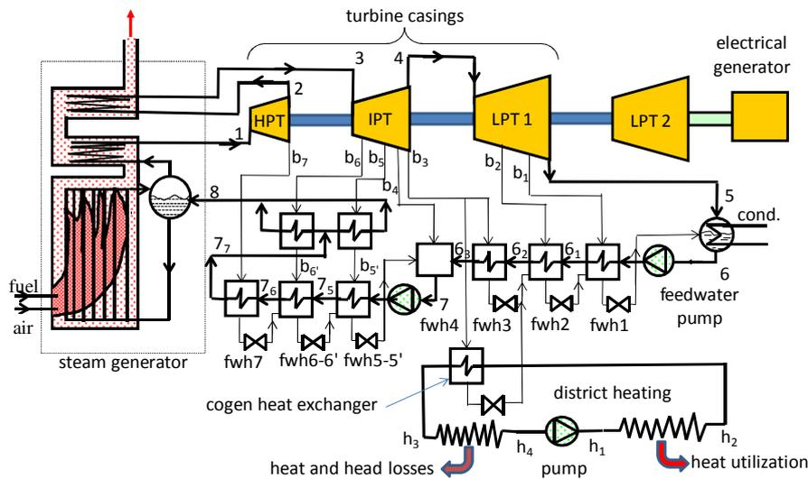
Fig. 5. Operating layout of the plant without second LP turbine and with cogeneration
