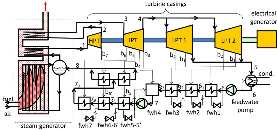
Fig. 2. Reference power plant layout
