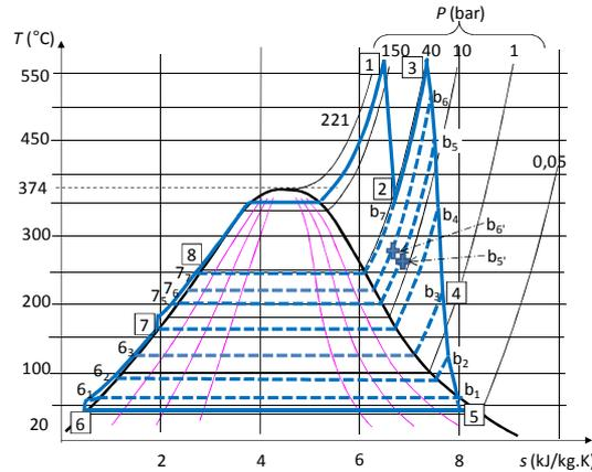
Fig. 3. Cycle characteristics in the entropy diagram
