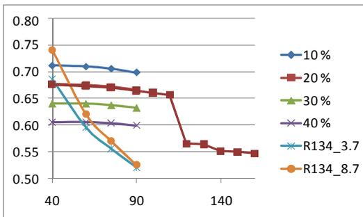
Fig. 7. Overall thermal + power generation efficiency depending on the heat temperature in cogeneration and heat pumps
