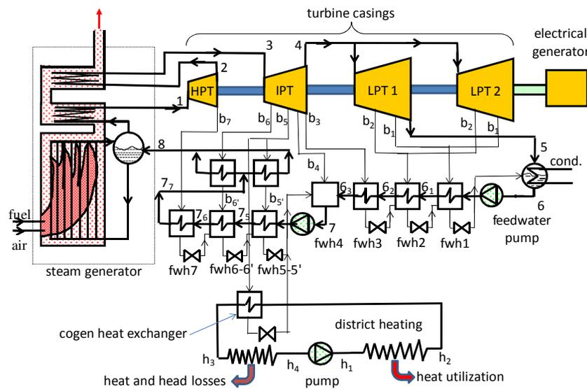
Fig. 6. Operating layout of the cogeneration power plant with  $b_5$  heat extraction
