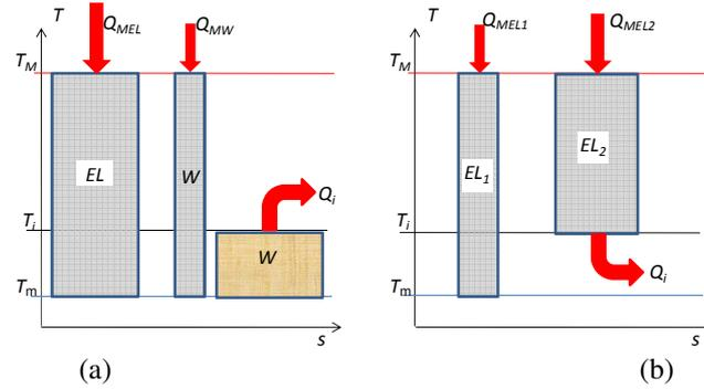
Fig. 1. Production of electricity and heat: (a) heat pumps, (b) cogeneration
