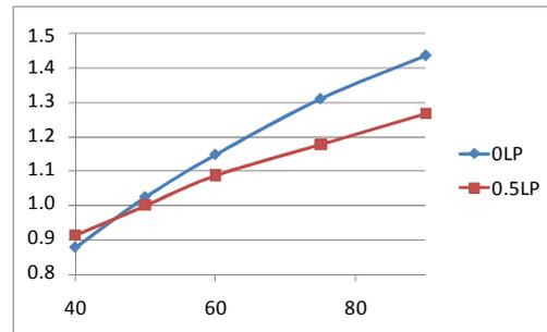
Fig. 8. Ratio of overall efficiencies CHP / heat pumps in the case of half LP production (0.5LP) and zero production (0LP)
