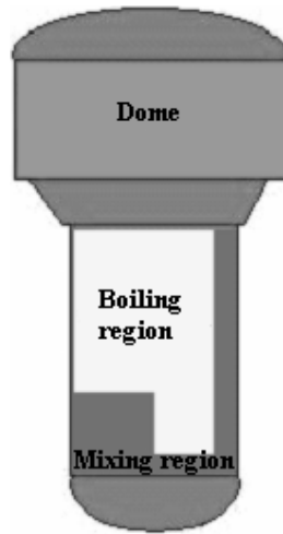
Fig 2. Secondary circuit dividing scheme
