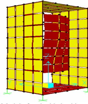
Fig. 6. Model of embedded cabinet. Cabinet with included strengthening bars. Mode 1 of vibration with  $T = 0.23s$  belong to panels on which the equipment is installed.
