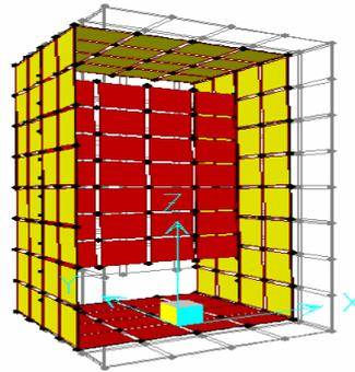
Fig. 8. Model of seismically isolated cabinet. Vibration mode 2. Left-right movement.
