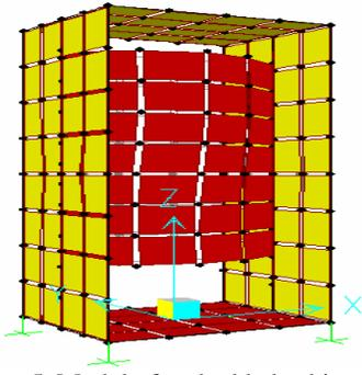
Fig. 5. Model of embedded cabinet. Cabinet without included strengthening bars. Mode 1 of vibration with  $T = 0.3s$  belongs to panels on which the equipment is installed.
