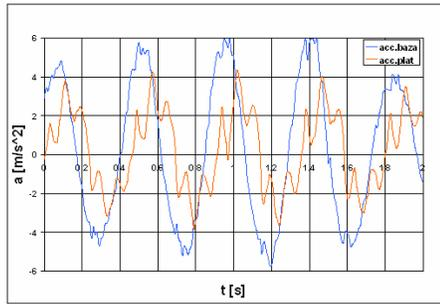
Fig. 12. Horizontal excitation and response accelerations of SERB mechanical device for a 20 kg mass.
