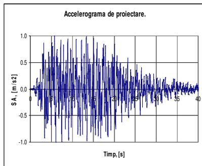
Fig. 3. Seismic design acceleration time-history.
