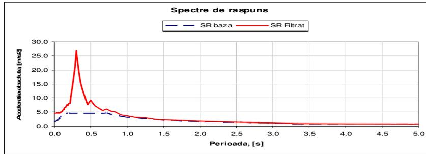
Fig. 9. Response spectra associated to the acceleration time-history used for equipment placed at ground and superior floors.
