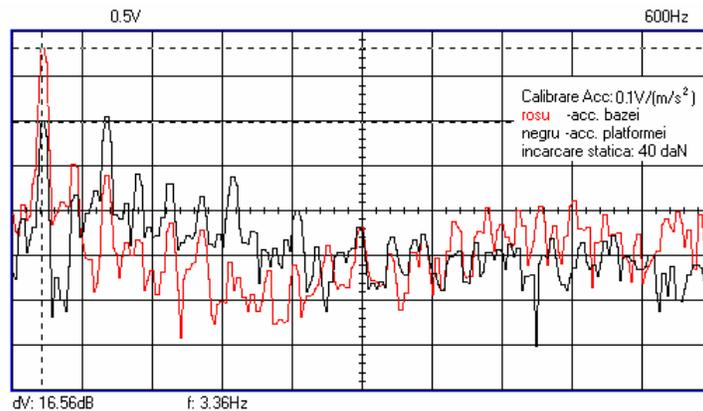
Fig. 14. Acceleration-frequency spectra model for input and output SERB device for a 40 kg attached mass.
