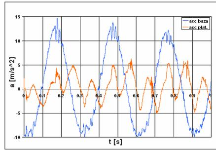
Fig. 13. Horizontal excitation and response accelerations for SERB mechanical device for a 40 kg mass.
