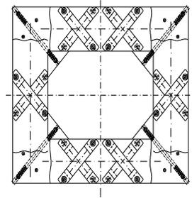
Fig. 2. SERB 1000/800 seismic isolation mechanical device.
