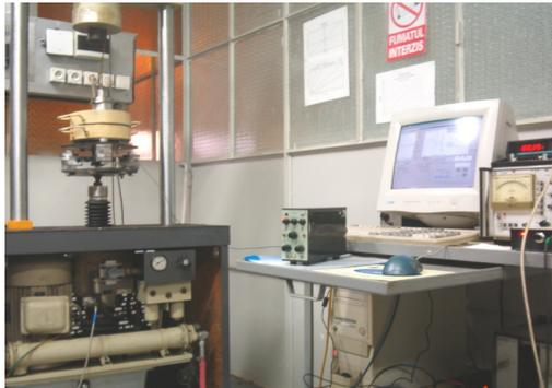
Fig. 10. Model of SERB 1000/800 device. Dynamic tests on the horizontal plane for the determination of the “cutting” capacity of the seismic acceleration.
