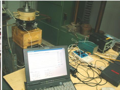
Fig. 11. Model of SERB 1000/800. Dynamic tests on the vertical direction for the determination the dynamic response of the device – additional mass and stiffness.
