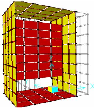
Fig. 7. Model of seismically isolated cabinet. Vibration mode 1. Back-front movement.
