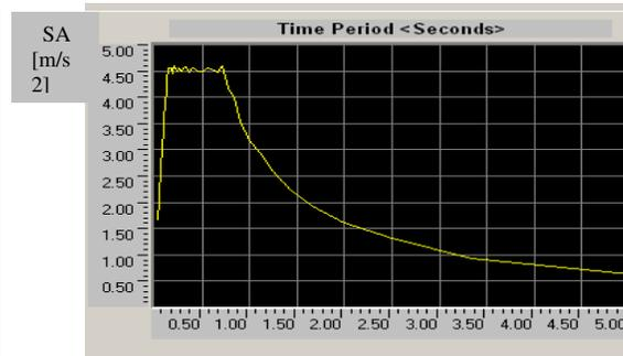
Fig. 4. The response spectrum of the location corresponding to the design acceleration time-history.
