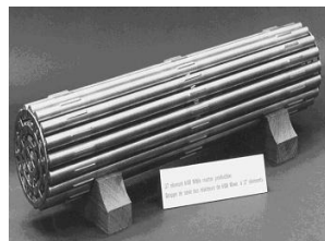
Fig.1. CANDU 600 Standard 37 fuel rods bundle. Side view of PT, rods, spacers and bearing pads.
