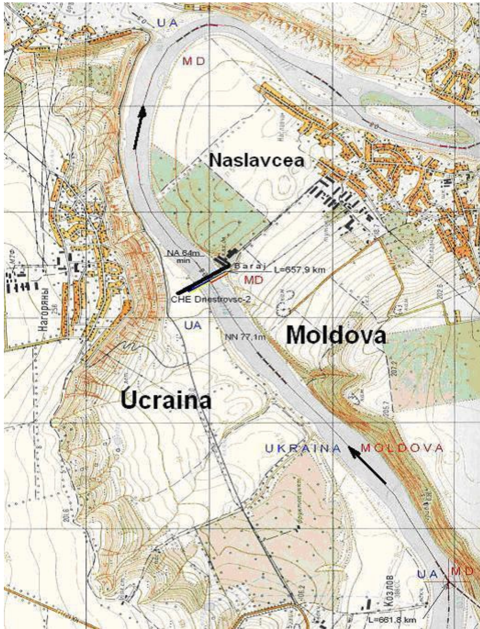
Fig.5. The plan of a site of the river Dniestr in north Moldavia (Naslavcea) with a dam by buffer hydroelectric power station Dnestrovsc-2 and zone of length 3,9 km in the top part of reservoir belonging Moldavia as well as and half of dam with hydrotehnical structures
