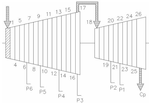
Fig. 1 DKUL 50-1 Counter-pressure steam turbine
