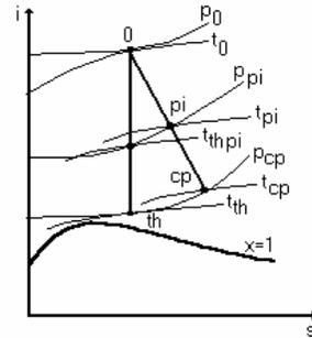
Fig.2 i-s diagram for the running cycle of a counter-pressure turbine with an adjustable mash.
