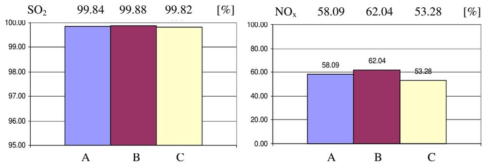
Fig. 5. SO<sub>2</sub> and NO<sub>x</sub> retention factor for the 3 types of fuel (agricultural biomass with pit coal)
