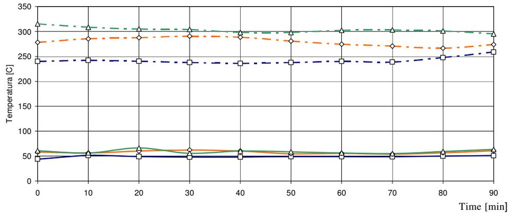
Fig. 4. Temperatures variation before and after the flue gas cleaning system (FGCS) for the 3 types of fuel (agricultural biomass with pit coal)
