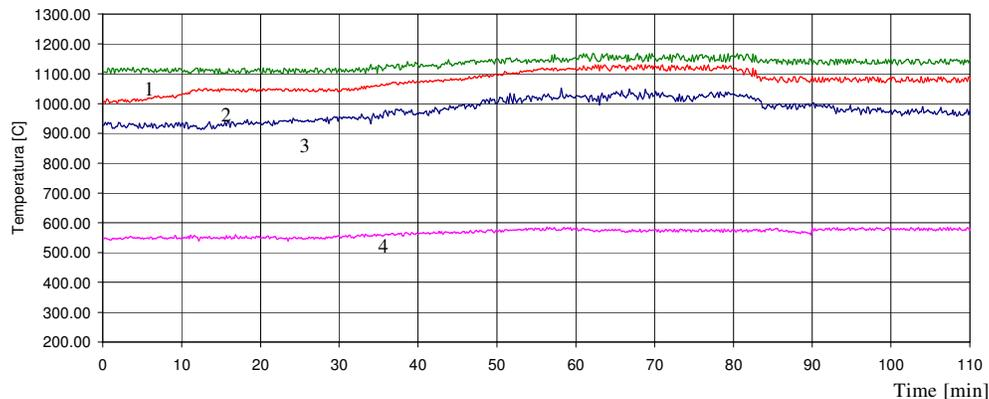
Fig. 3. Temperatures variation in furnace and convective case for approx. 2 hours of running with maize and pit coal
