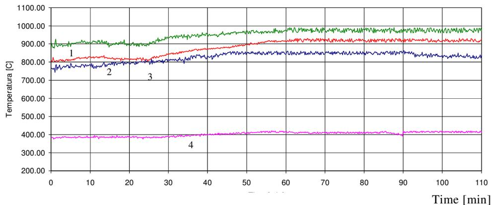
Fig. 2. Temperatures variation in furnace and convective case for approx. 2 hours of running with corncob and pit coal
