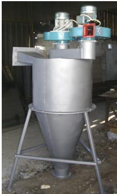
Fig. 2.1 Prototype of a modular system for industrial gas depollution – General View
