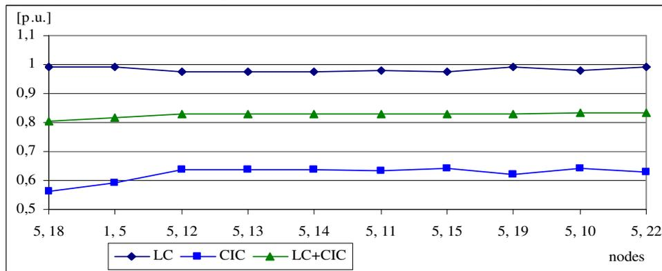
Fig. 6. Costs variation (in p.u.) for two  $DGs$  considering uniform consumption at nodes.
