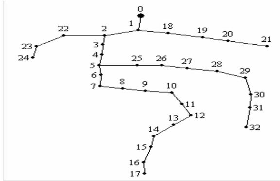
Fig. 2. Electrical network with 33 buses and 32 branches.
