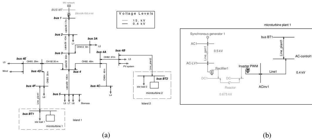
Fig. 3. Test system (a) and a detail of the microturbine system for plant 1 (b)
