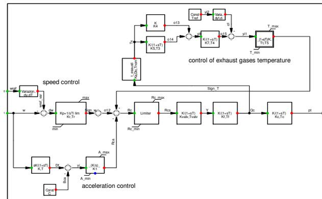
Fig. 2. Detailed scheme of the microturbine with relevant controls (acceleration, speed and temperature control)
