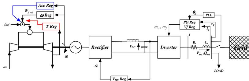
Fig. 1. Microturbine based generation plant with its control loops
