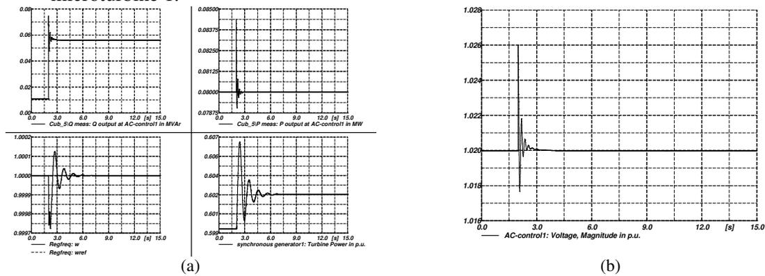
Fig. 5. (a) Reactive and active power of inverter 1, speed and turbine power for microturbine 1; (b) Voltage magnitude at the controlled bus in plant 1
