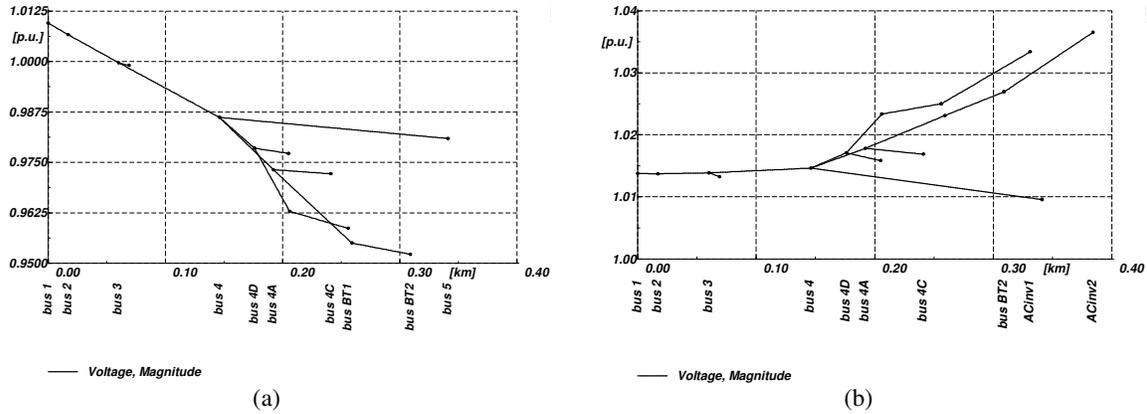
Fig. 4. Voltage profile along the feeders of the LV distribution network: (a) without microturbine plants; (b) with microturbine plants
