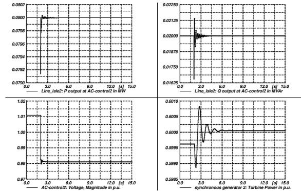
Fig. 6. P and Q of inv. 2, voltage magnitude at AC-control2 and turbine power of microturbine 2
