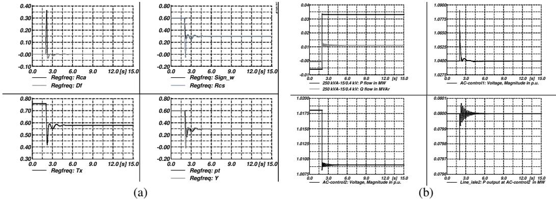
Fig. 7. (a) Mechanical quantities related to microturbine 1; (b) P and Q flow along the MV-LV transformer, voltage magnitude at AC-control1 and AC-control2, P output of inverter 2
