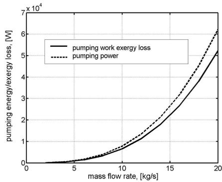
Fig. 1. Pumping energy/exergy loss vs.  $\dot{m}$
