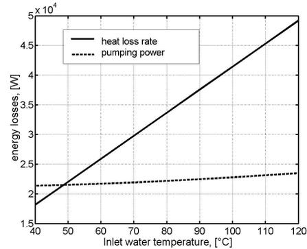
Fig. 6. Energy losses vs.  $T_s$
