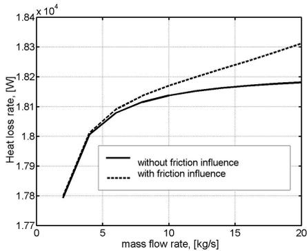
Fig. 3. Heat loss vs.  $\dot{m}$
