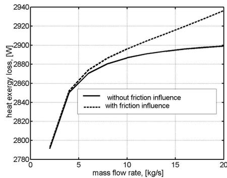
Fig. 4. Heat exergy loss vs.  $\dot{m}$
