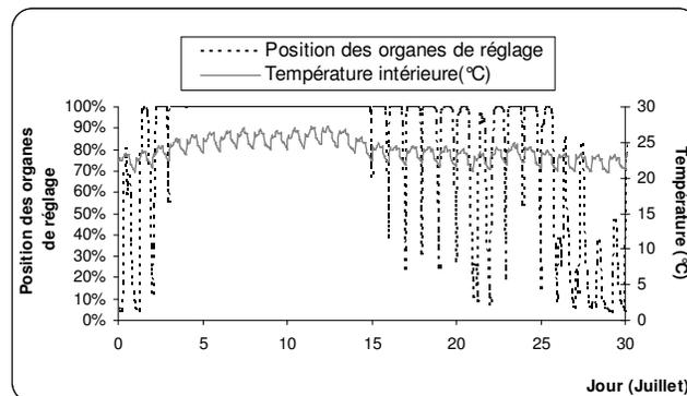
Fig. 7. Mixing rate “chilled water / cooling coil outlet water” as a function of indoor air temperature
