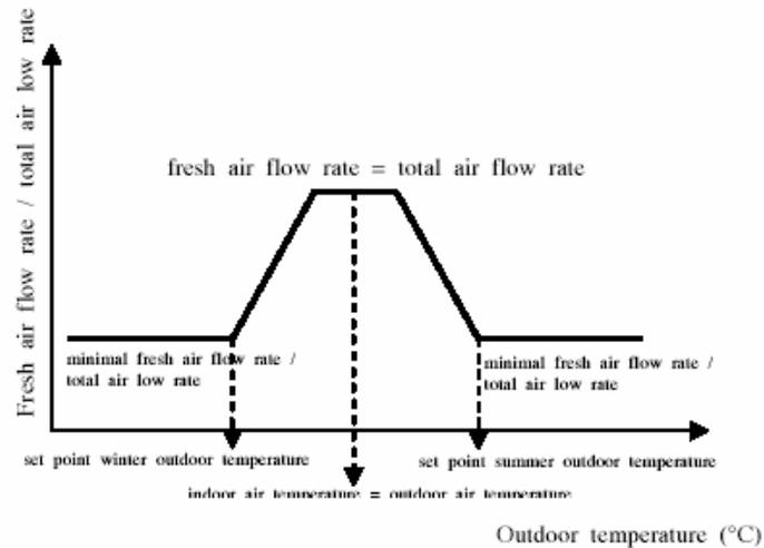
Fig. 3 Fresh air modulation as a function of outdoor temperature
