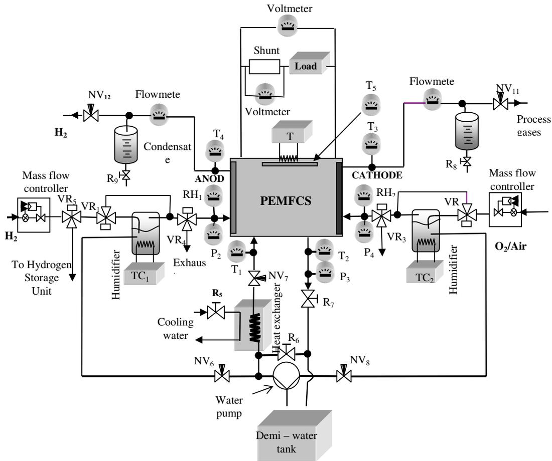
Fig. 2 Fuel cells stack fluid management schematic
