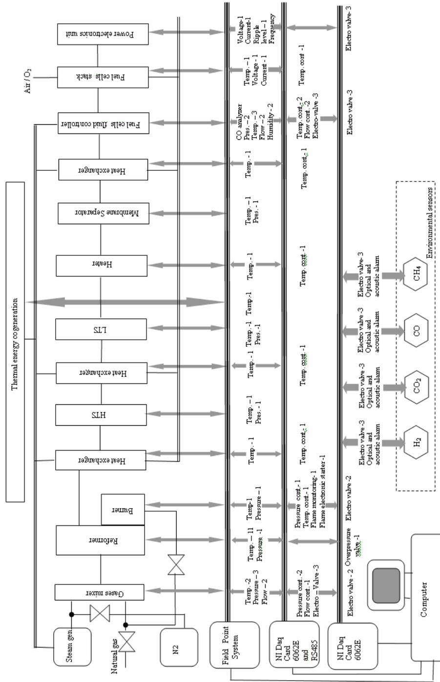
Fig. 1 Schematic of the energy conversion pilot plant controlling system
