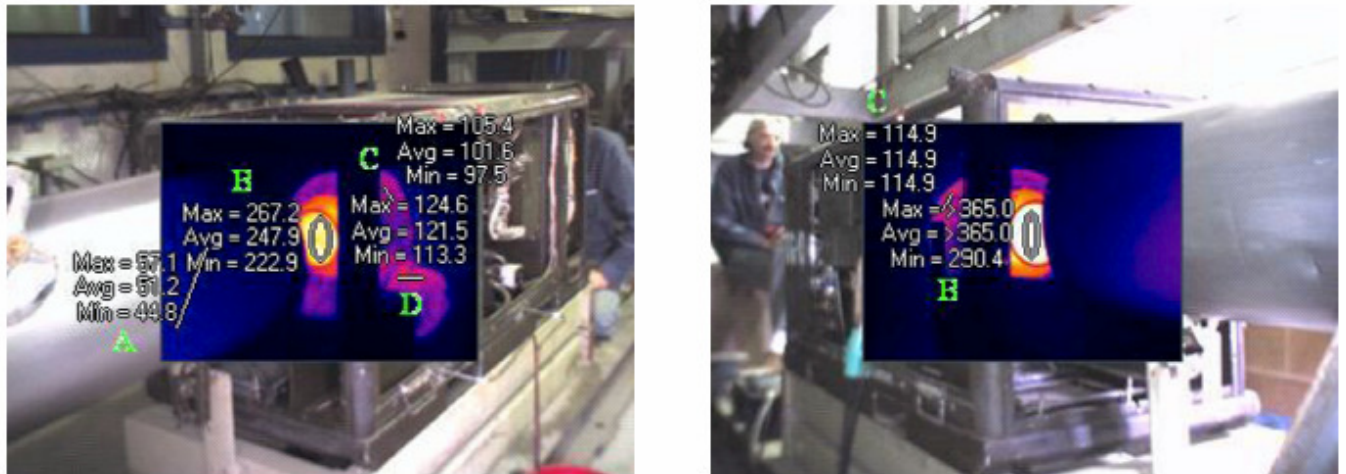
Figure 7: Infrared view of the Garrett 30-67 engine exhaust nozzle
