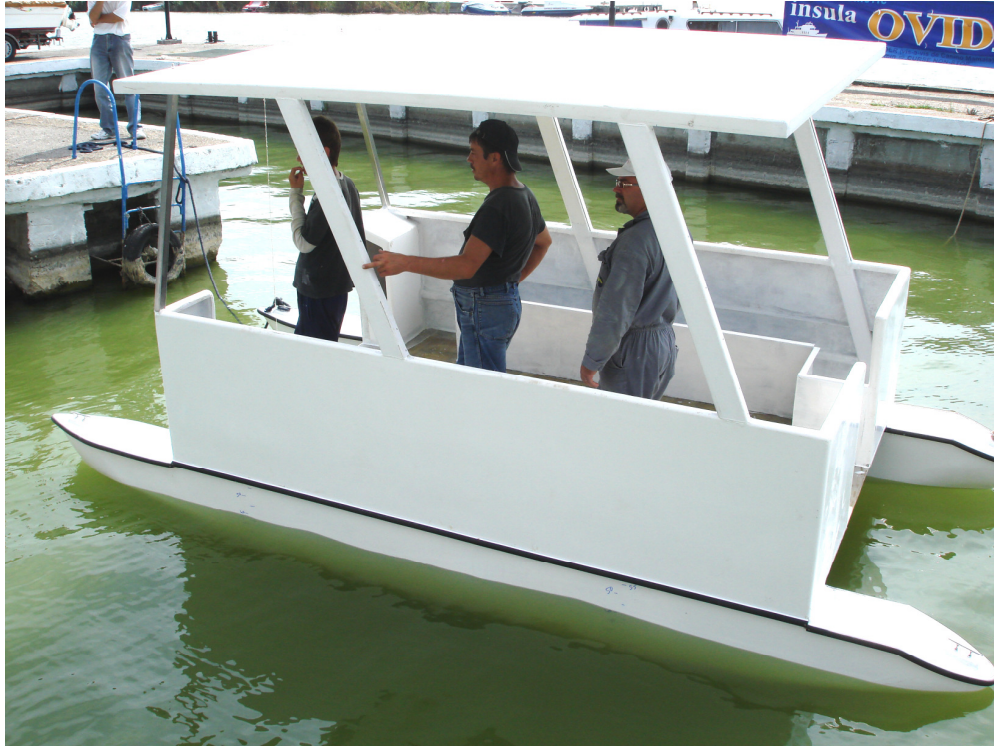
Fig. 1. Aspect of the realised ecological boat of catamaran type
